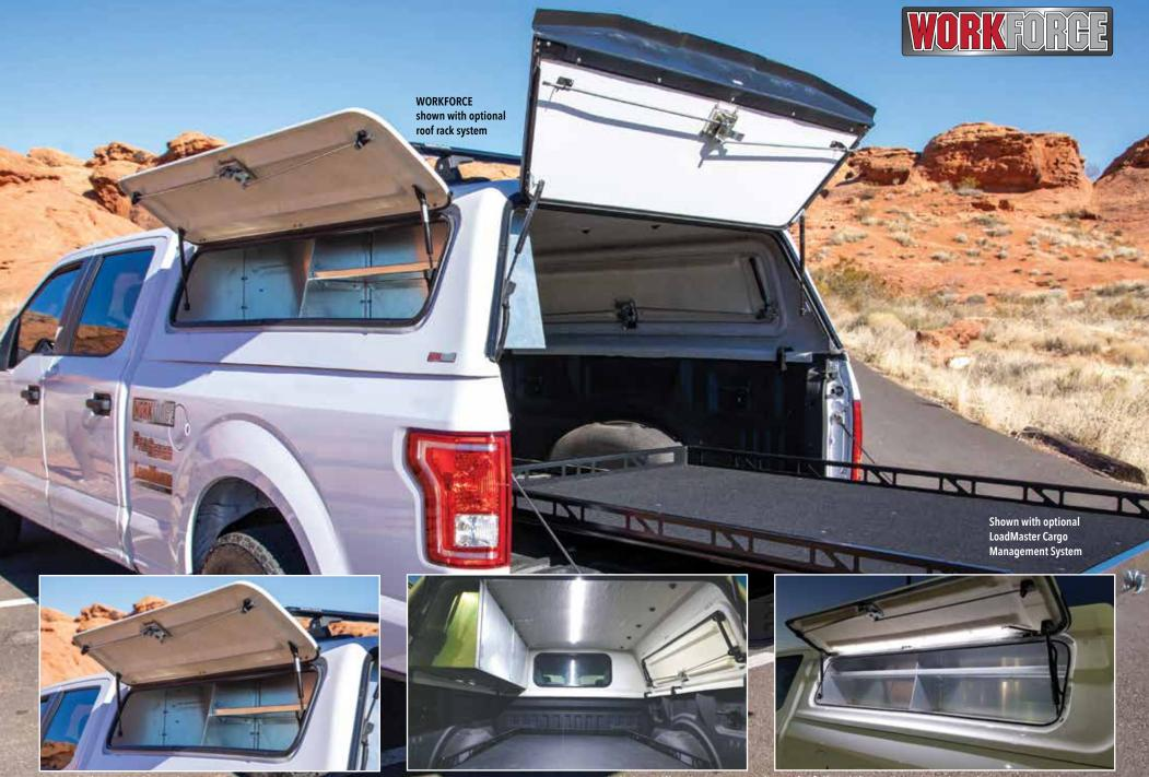
3 point locking side doors, shown with galvanized steel tool boxes
