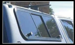
Optional side Windoor with Slider provides ventilation without opening the entire Windoor
